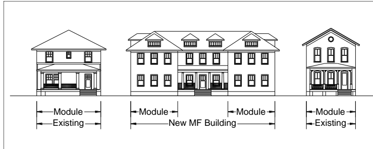
Building modules that break up the horizontal plane
