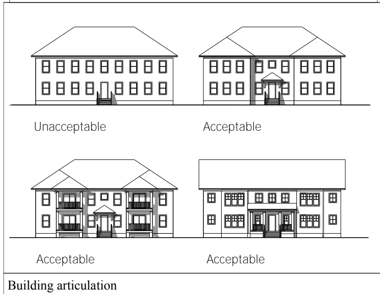
Building modules that break up the horizontal plane
