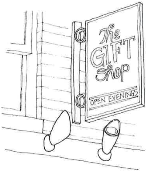
Lighting should be shielded and directed toward a sign to avoid glare.
